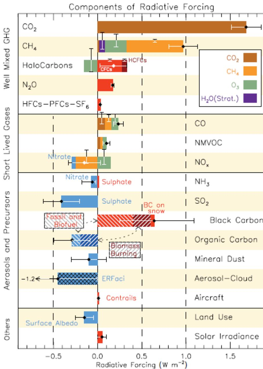
Figure 4 The components of climate forcing at global scale. Source: IPCCAR5 WG 1 fig 8.7 (Myhre et al 2013)
