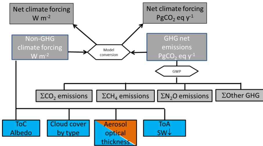
Figure 5 The top-level components of an anthropogenic climate forcing observation system from Africa. Shades of grey are observationally-constrained model products. Sky blue is for space-based observations, orange-brown is for land-based observations. Abbreviations are tabulated at the end of the report.
