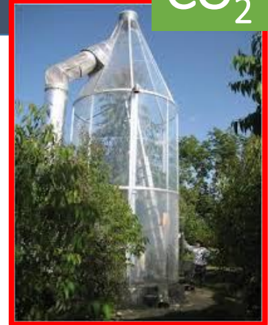
Whole-Canopy gas exchange chamber (CO 2 , H 2 O – ANPP & T)
