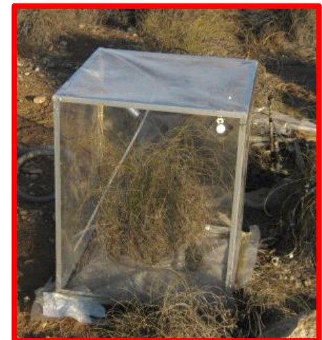
Whole-Canopy gas exchange chamber (CO 2 , H 2 O – ANPP & T)
