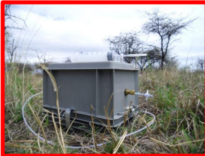
Chamber method ( \text{CO}_2 , \text{H}_2\text{O} – NEE & ET plot scale)
