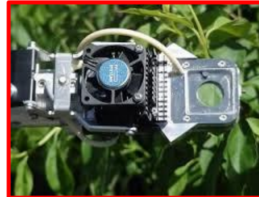
Leaf gas exchange sensors (CO 2 , H 2 O – ANPP & T)
