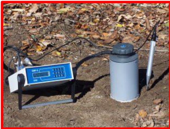
Chamber method ( \text{CO}_2 , \text{H}_2\text{O} – R_{\text{soil}} & E, soil efflux)
